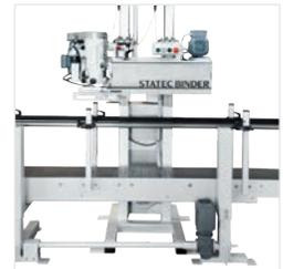
The high-performance sewing machine from STATEC BINDER closes woven polypropylene, paper and polyethylene bags accurately and securely.
